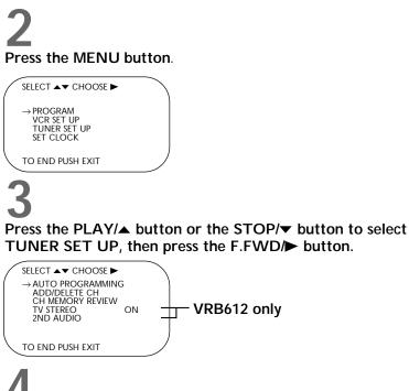
Press the PLAY/▲ button or the STOP/▼ button to select AUTO PROGRAMMING, then press the F.FWD/▶ button. The VCR distinguishes between TV channels and cable channels, and the VCR will memorize all the channels you receive.
